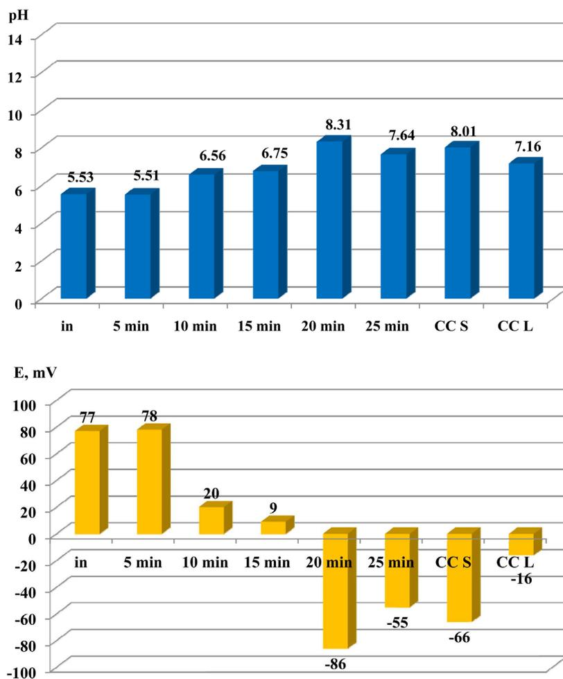
**Figure 4.** Variation of pH values and redox potential ( $E$ , mV) when electroactivating undiluted RBY (C1).  $j = 20 \text{ mA/cm}^2$ ; CC S—Cathode cell content (foam phase); CC L—Cathode cell content (liquid phase).
