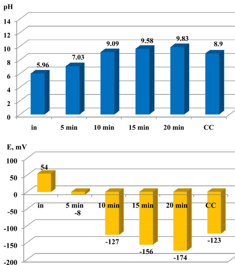
**Figure 6.** Variation of pH and redox potential (E, mV) values at 1:3 diluted RBY electroactivation (C2).  $j = 20 \text{ mA/cm}^2$ ; CC S—Cathode cell content (foam phase); CC L—Cathode cell content (liquid phase).
