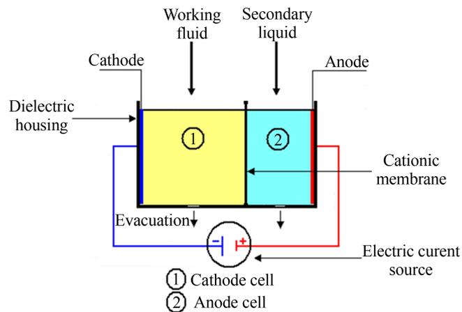
**Figure 2.** Scheme of the EDP-0.5 diaphragm electrolyzer.
