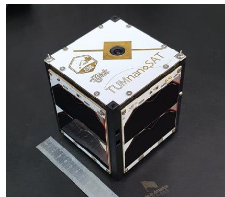
Figure 1. TUMnanoSAT the first TUM 1U CubeSat
