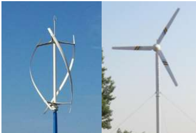
Figure 1. VAWT (Quiet Revolution) and HAWT (Technical University of Moldova).
