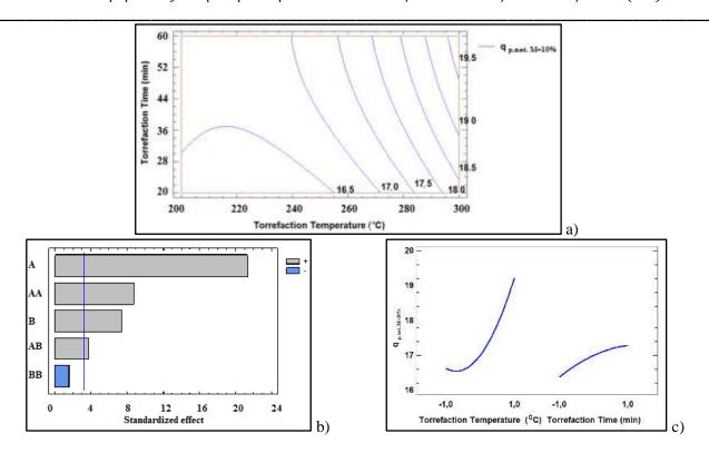
Figure 2. Calorific value of the biomass mixture that includes 50% of blackberry, 50% of sea buckthorn according to torrefaction temperature and time:
