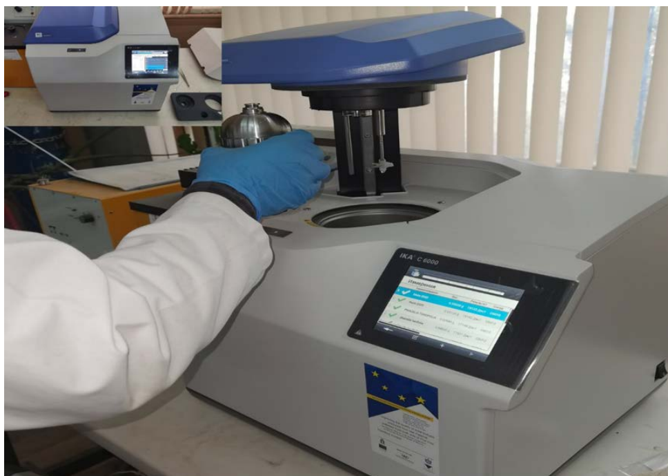
Figure 3. Determining the gross calorific value by IKA C6000 isoperibolic calorimeter in the Solid Biofuels Laboratory, SAUM.
