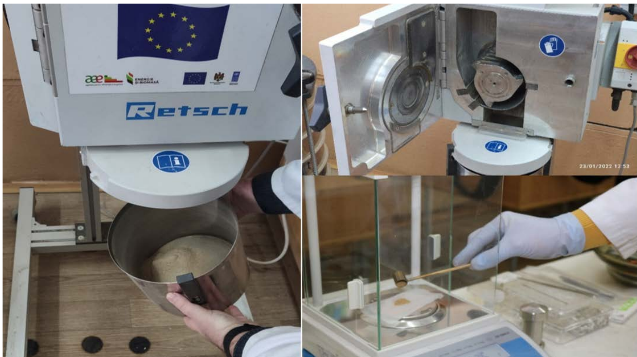
Figure 4. Pellet crushing and sample dosing by weighing.
