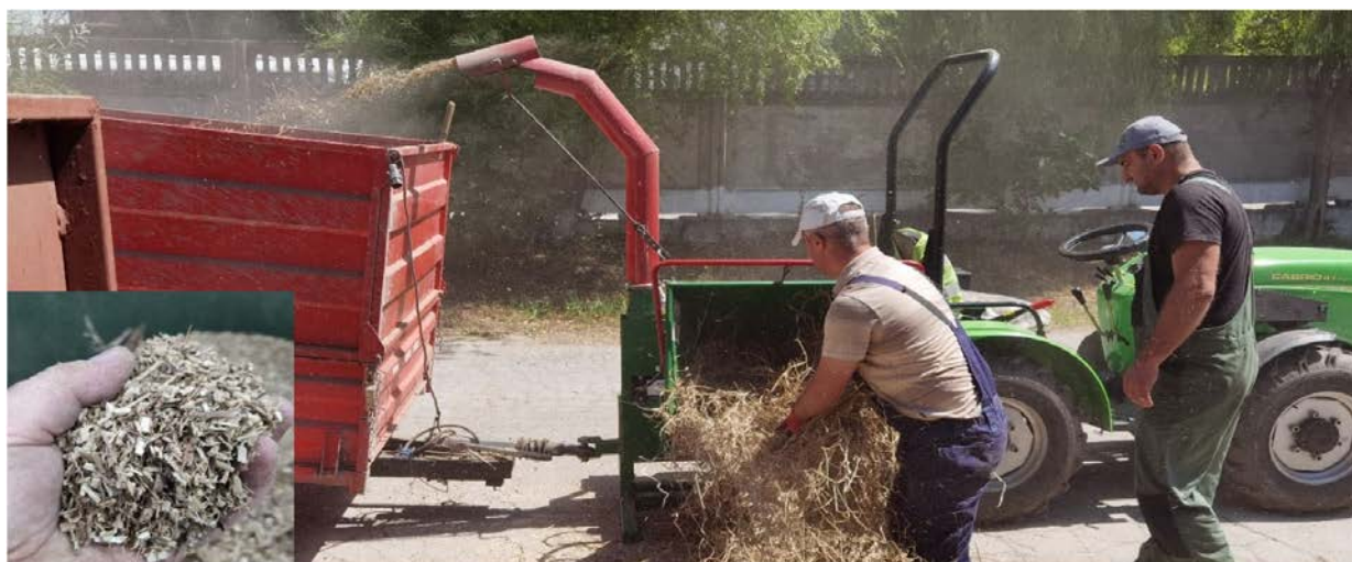
Figure 1. Coarse shredding of Miscanthus biomass using Murena shredder attached to the MT 8E2 tractor.
