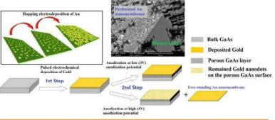
Schematic representation of the technological route for the fabrication of Au nanomembrane on a porous semiconductor substrate with possibilities to be transferred to another substrate. Inset is the illustration of the mechanism of hopping electrodeposition of a monolayer of Au nanodots and SEM image of an Au nanomembrane prepared by electroplating with pulse duration of 300 µs.
