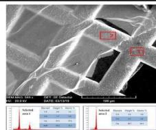
EDX analysis of an Au nanomembrane transferred to a TEM grid.
