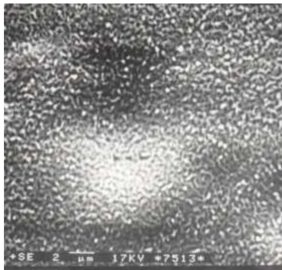
Figure 1. SEM micrographs of Te grown on Pyrex with on deposition rate v = 1 nm/s
