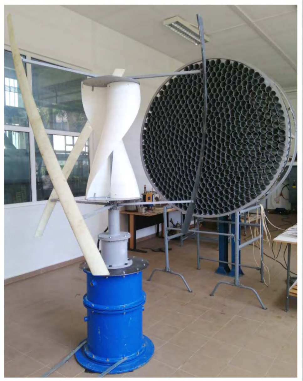
Experimental prototype of vertical axis wind turbine designed, manufactured and researched experimentally at UP Bucharest
