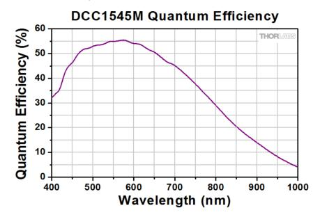
Figure 4. Quantum efficiency of the DCC1545M CMOS camera.
