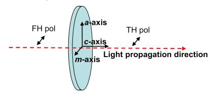
**Figure 5.** Schematic representation of crystallographic *a*, *c*, and *m* axes relative to the investigated GaN sample plane. The light propagation direction and its polarization are also shown.
