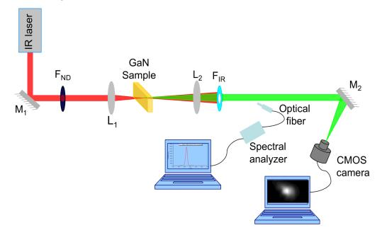
Figure 3. Schematic of the experimental setup used for THG in GaN crystal.
