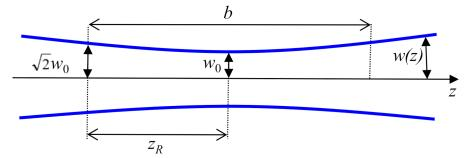
Figure 2. A schematic of the Gaussian beam propagation near the focus of a focusing lens.
