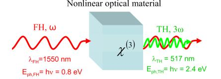
Figure 1. A graphical illustration of the THG process.
