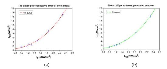
**Figure 8.** The experimental curves  $I_{\text{TH,peak}}(L) = f(I_{\text{FH,peak}}(0))$ , considering the entire photosensitive array of the camera (**a**), and a 200 px \* 200 px software generated window surrounding the measured beam spot (**b**), respectively.
